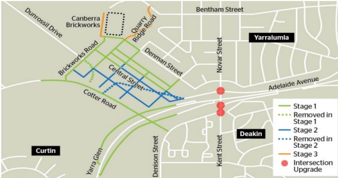
A diagram showing roads planned for the redevelopment, with part of Dunrossil Drive and Dudley Street (dotted) to be removed.
